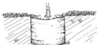
Figure 11. Mulch shall taper to a slightly thinner layer on top of the root-ball.
